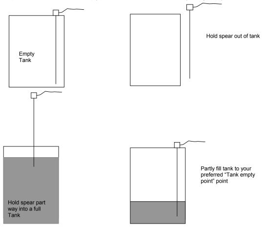
Please Note: The true EMPTY point is the level of the pump-out pump fitting as it can never be emptied below this point.
