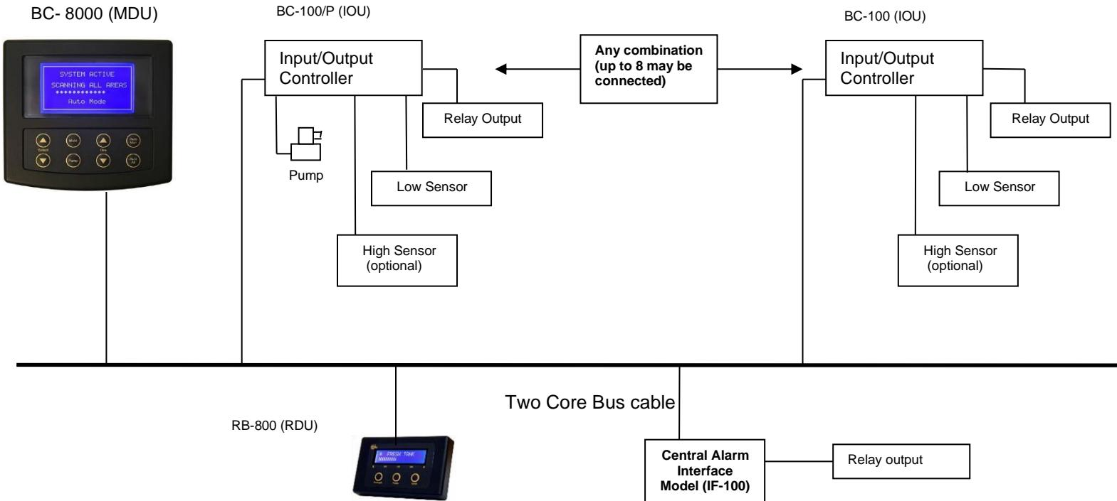
**Note:** The Central Alarm Interface is an optional extra and provides the ability to spy on the network for any data e.g. any High Sensor On, any Pump On, which may be required as an input for another device. The IF-100 has one Relay output.
