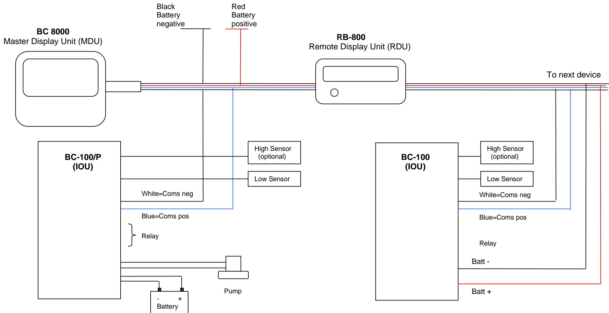
**WARNING:** As the BC-100/P supplies power for the pump, the supply cables & fuse need to be rated as per the pump manufacturer's specifications.
