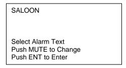
Use the Select Up or Down key to scroll through the pre-named zone names. Once you have found the one required press the Ent key.
