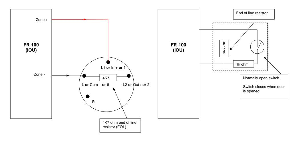
**Note:** Detector manufactures use different terminal designators, E.g. L1, L2, L3 **OR** Com – , In + , Out + **OR** 1, 2, 3, 4, 5, 6
