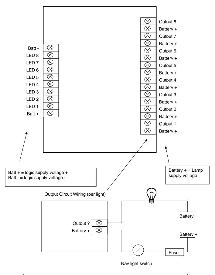
**NOTE:** If a single switch is used to turn all the nav lights ON and OFF then simply loop all the Battery + terminals together
