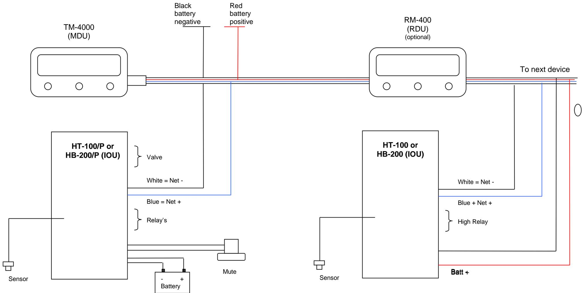
**WARNING:** As the HT-100/P & HB-200/P supply power for the pump, the supply, cables & fuse need be rated as per the pump manufacturers specifications.
