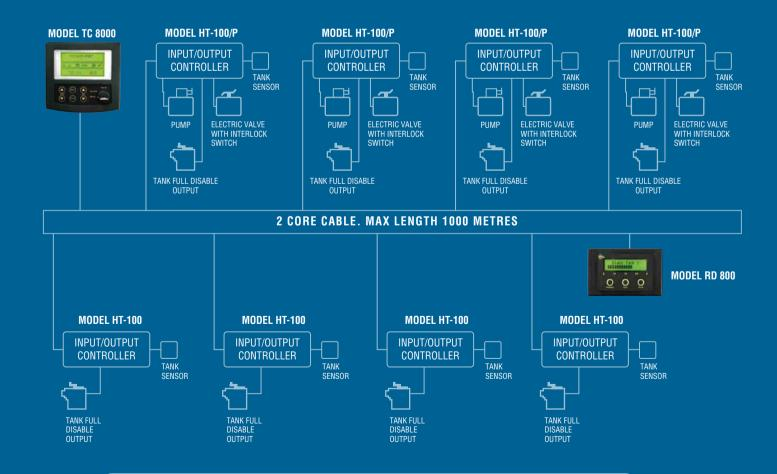
Supply Voltage: 12 ~ 32 Volts DC (Auto sensing) | Quiescent Current: 5 Milliamps (without backlight)
