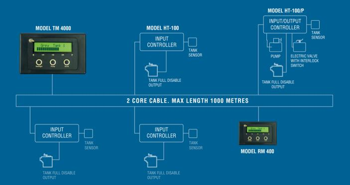
Supply Voltage: 12 ~ 32 Volts DC (Auto sensing) | Quiescent Current: 5 Milliamps (without backlight)
